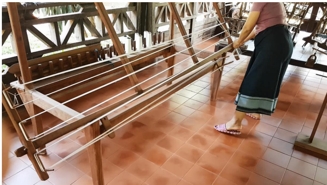
Figure 22: Warping procedure shown in the Lao Textiles Museum, Vientiane 160
