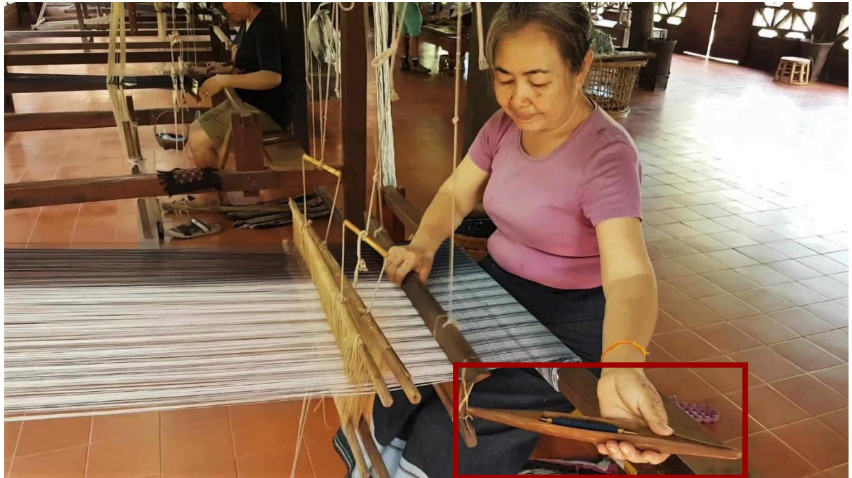
Figure 30: Bouavanh Phouminh inserts the weft threads by moving a shuttle , which contains a bobbin of yarn, through the shed
