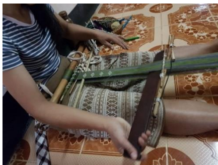
Figure 24: Opening a shed, Luang Prabang
