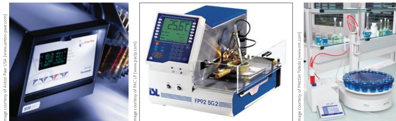
Figure 1 —Typical instruments for measurement of density and viscosity, flash point, and total acid number (left to right).
