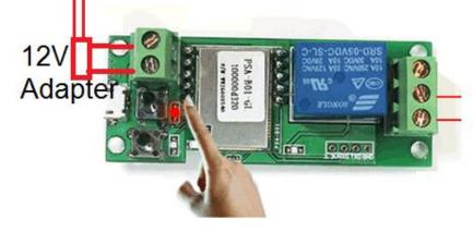
Connect these wires either to the wall switch terminals of the main unit opener or directly to the wall switch
