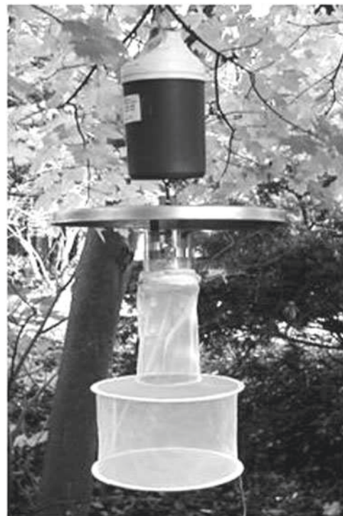
FIG. 4. Carbon dioxide light trap.
