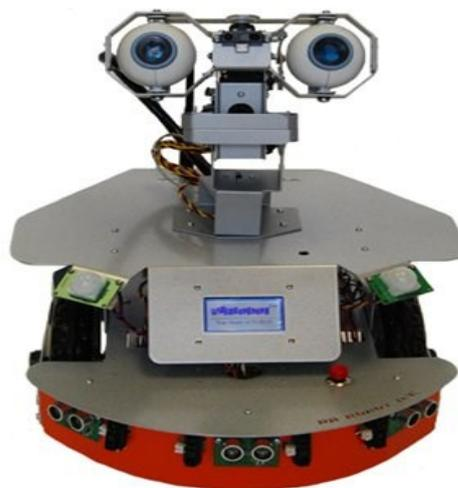
**Picture 3.23 Vision system in robot**
