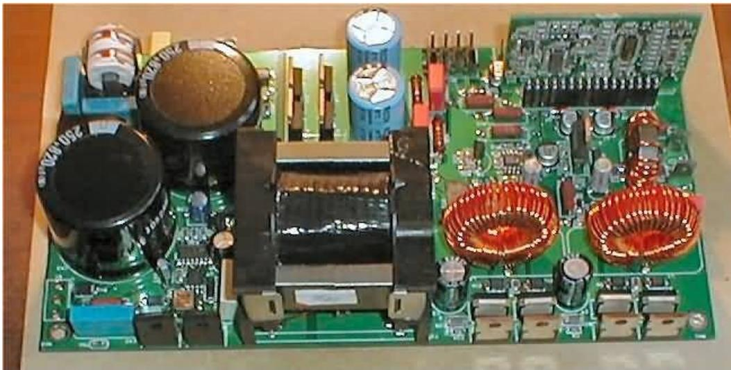
**Picture 3.6 Power supply circuit**
