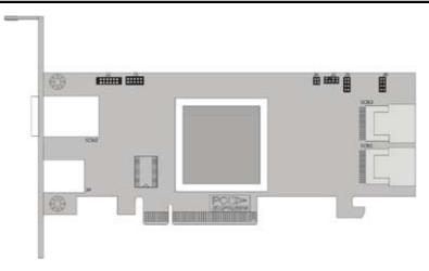
Figure 2-2, ARC-1680ix-8 Internal/External SAS RAID Controller
