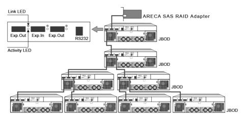
Figure 2-8, External connector to a drive box or drive enclosure
