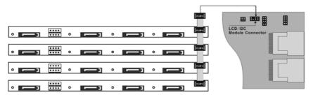
Figure 2-20, Activity/Fault LED I<sup>2</sup>C connector connected between SAS RAID Controller & 4 SATA HDD backplane.
