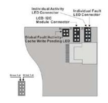
Figure 2-18, ARC-1680i individual LED for each channel drive and global indicator connector for computer case.
