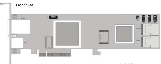
Figure 2-5, ARC-1680IXL-12/16 SAS RAID Controller
