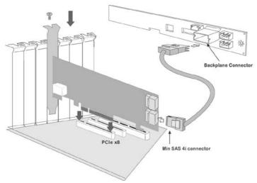
Figure 2-10, SAS Cable Connect to Backplane
