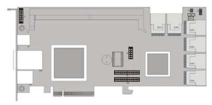
Figure 2-1, ARC-1680ix-12/16/24 SAS RAID Controller
