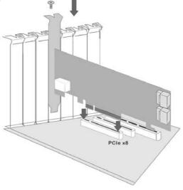
Figure 2-7, Insert SAS RAID controller into a PCIe slot
