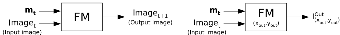
Figure 5.1 — Left: Visual forward model (FM). Right: Single component of a visual forward model predicting the intensity of a single pixel (x_{\text{Out}}, y_{\text{Out}}) of the output image (adapted from Schenck and Möller, 2007 , © Springer).
