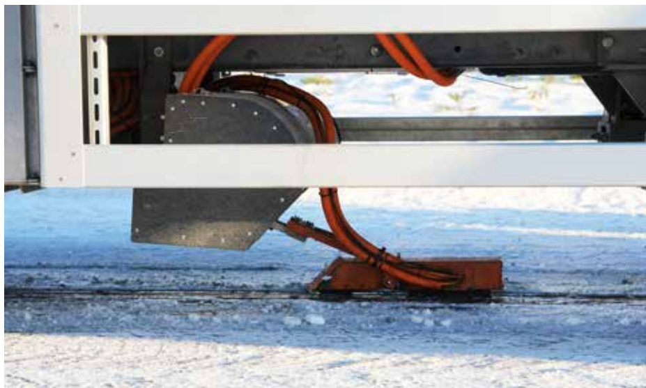
An arm under the truck, eRoadArlanda.
