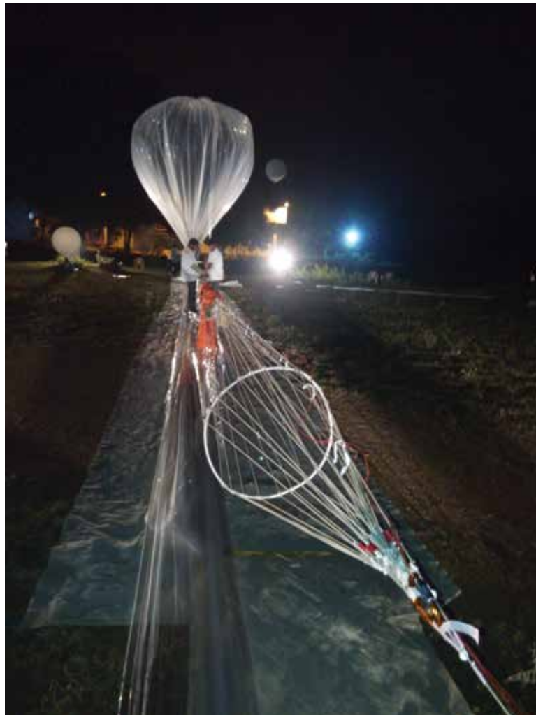
Zero pressure balloon (3026 cu.m.) after bubble inflation with a parachute prior to launch during Batal campaign (13th Aug 2015)
