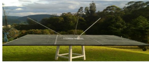
Fig 10: The 70 MHz monopole antenna configuration with a ground-plane, ready for experiments at the test range at the Radio Astronomy Centre, Udhagamandalam
