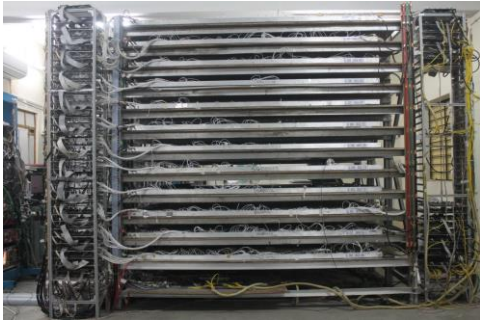
Fig: 2: 2m x 2m RPC detector stack in operation at IICHEP, Madurai
