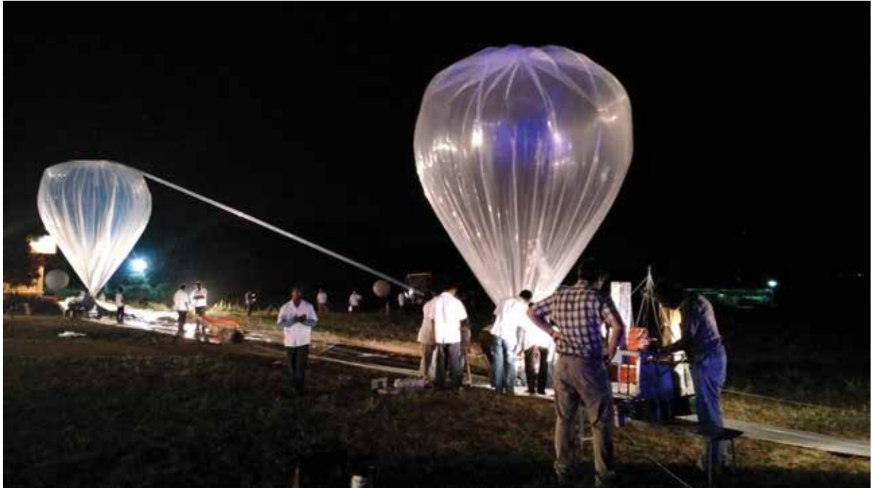
Zero pressure balloon (300 cu.m.) along with an auxiliary balloon ready for launch for carrying an atmospheric science payload during NARL-NASA-University of Wyoming's Batal campaign (July-August 2015)
