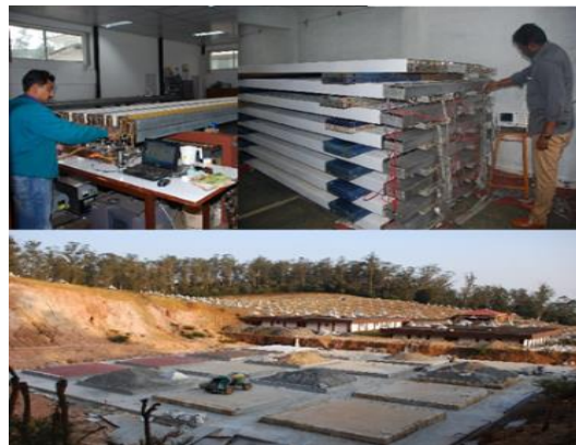
Figure 5: Pictures on upper panel show PRC fabrication and testing. Lower panel shows platforms for new muon detector.
