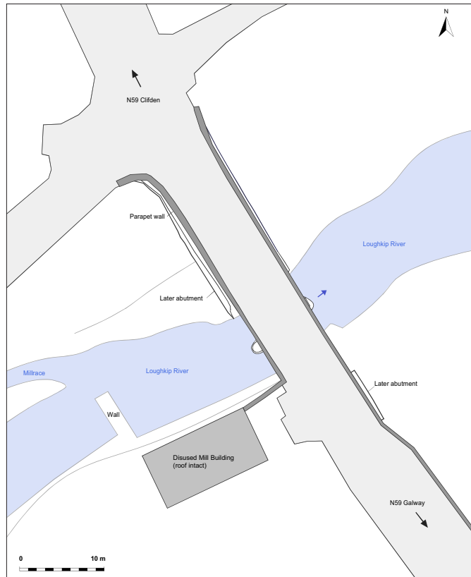
Illus. 1.31 (above)—Measured survey drawings of the south-west (upstream) and north-east elevations of the old Clydagh Bridge on the Lough Kip River; on the eastern approach to Moycullen on the N59; and (right) a plan of the bridge, showing also the adjacent Victorian grain mill. The relieving arches on the upstream side suggest rebuilding of that façade and this may have been the work carried out by Alexander Nimmo in 1829. The different treatments of the parapet walls also suggest rebuilding. The massive rubble masonry cladding of the abutments is a more recent addition. The bridge was probably built in the mid-18th century by the Galway Grand Jury (precursor to the local authority until 1898). It was demolished and replaced in 2015–16. ( Hugh Kavanagh for Irish Archaeological Consultancy Ltd )
