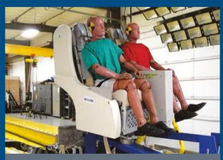
PAC'S 58" PITCH DOUBLE SLEEPER SEAT BEING Dynamically tested for Faa Certification
