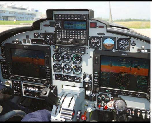
Up-front control (top, centre) and two large multi-function displays – state of the art.
