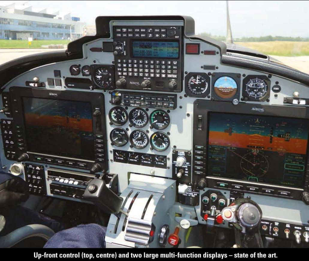
Up-front control (top, centre) and two large multi-function displays – state of the art.
