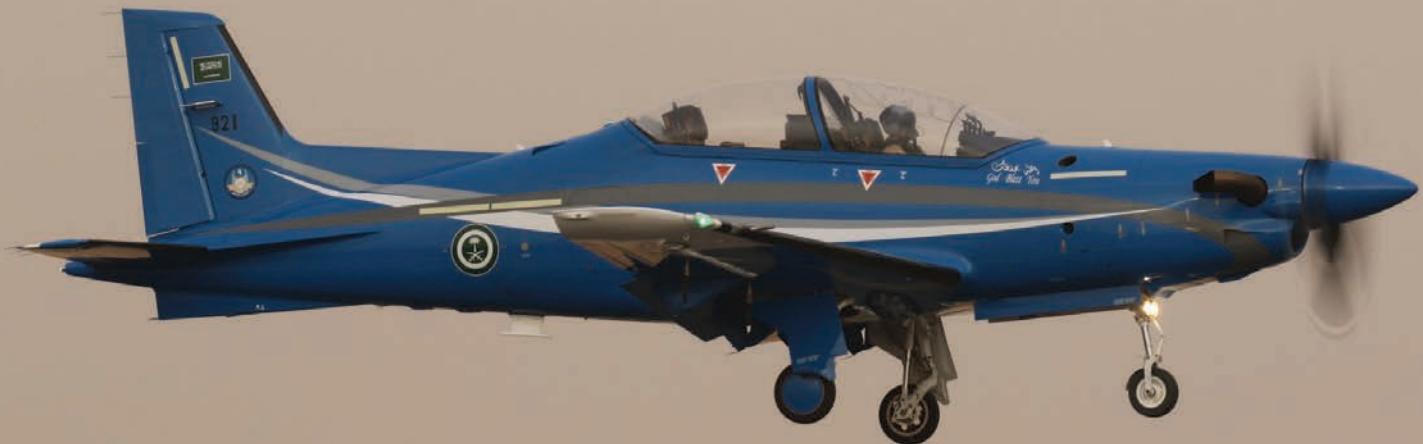
Like many Middle East air forces, the Royal Saudi Air force has opted for the Pilatus PC-21 in the basic/advanced flying training role.
