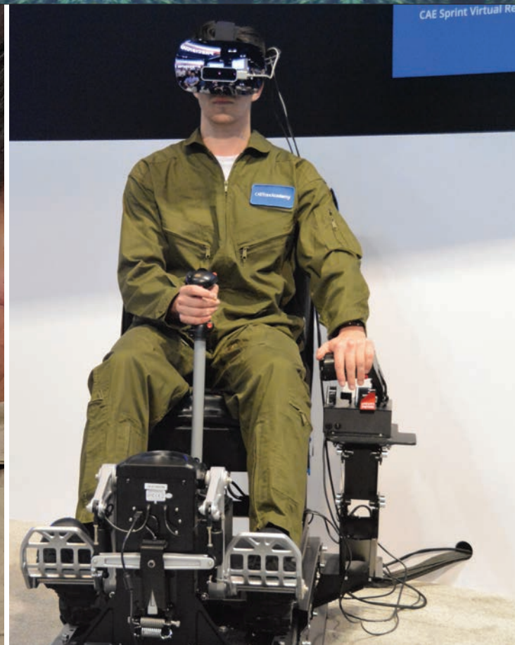
The CAE Sprint virtual reality trainer with a student pilot. He is seen wearing a VR headset, with a stick and control panel under his left hand.
