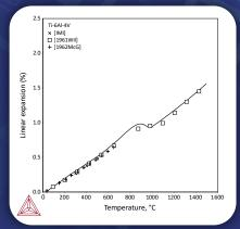
Linear expansion vs Temperature for Ti-6AI-4V
