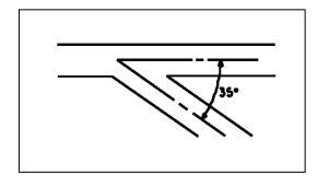
For roadway approaches with line of sight angles less than 35 degrees, use full-circle signal head visors with visibility-limited signal devices.
