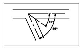
For roadway approaches with line of sight angles between 35 degrees and 65 degrees, use tunnel signal head visors or full-circle signal head visors.
