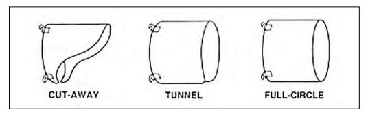
Cutaway visors, sometimes referred to as a cap or partial visors, are signal head visors with the bottom cut away. This type of signal head visor reduces water and snow accumulation and does not let birds build nests within the visor.
