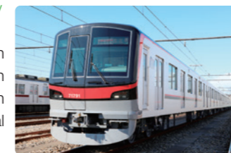
Lightweight aluminum alloy body
