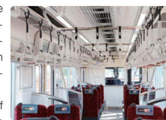
LED in-car lighting
