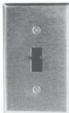
Operates both fan and room light. Fan powers on 15 seconds after light is turned on. Powers off 1 to 10 minutes after light is turned off. (Adjustable) Input: 120 VAC+ 10% 50/60 Hz, 3.5 watts max. Light: 3A resistive @ 120 VAC 500 watts max. Fan: 10A resistive, 1/3 HP @ 120 VAC.
