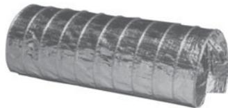
Features aluminum foil, fiberglass and aluminum polyester laminate construction. Pressure rated to +6" and -4" w.g. Rated velocity 4000 FPM. Operating temperature -20°F to 250°F. UL 181 Class 1 listed.
