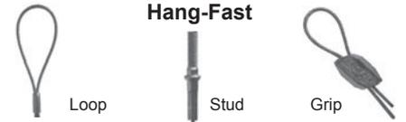
Provides lighter, easier and faster alternative to threaded rod for hanging mechanical, electrical and HVAC equipment. Ready to use; requires no additional preparation time. Includes cable with loop or stud end fixing; grip secures free end of cable and allows height adjustment of hanging object. **Loop.** For wrap-around anchoring on bar joists or other roof structures. **Stud.** For anchoring into concrete or metal. Includes 1/4" drop-in expansion anchor.
