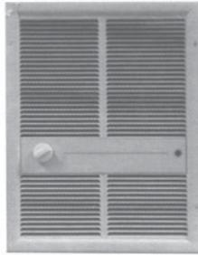
Constructed of heavy gauge steel with rough-in dimensions of 19-5/16" H x 14-3/16" W x 4" D. 600 RPM motor drives vane axial blower to deliver 175 CFM downflow air. Features standard thermal overload cutoff and built-in thermostat. Temperature range 55°F to 85°F. Ivory. UL listed.
