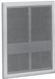
Constructed of heavy gauge steel with rough-in dimensions of 19-5/16" H x 14-3/16" W x 4" D. Grille measure 15-29/32" W x 20-27/32" H. 600 RPM motor drives vane axial blower to deliver 175 CFM downflow air. Features standard thermal overload cutoff, fan delay switch, automatic reset thermal limit switch and built-in thermostat. Temperature range 55°F to 85°F. Ivory. UL and CUL listed.
