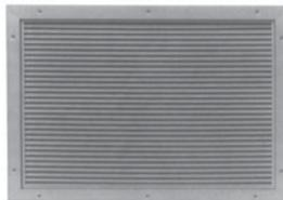
For use in doors and partitions. 20-ga. V-shaped steel blades block vision and increase strength. Countersunk screw holes for #8 sheet metal screws (included). Satin aluminum finish. Includes auxiliary frame.
