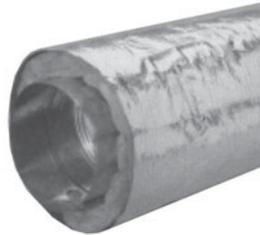
For use in air distribution systems, connecting ducts, room inlets or terminal devices. Puncture-resistant. Features flexible corrugated aluminum core with watertight lock seams, wrapped in fiberglass insulation blanket with metalized polyester jacket. Bends easily; maintains shape without sagging. Max. velocity 5000 FPM. 8-ft. length. R-value 4.2. UL 181 compliant.
