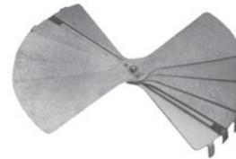
For use in flexible duct or where height is limited. Gang-operated design; blades slide at right angles to airflow. Mounts in diffuser neck, flush with top. Measures 1" D. Adjusts from face side of diffuser.
