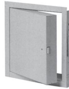
For vertical wall applications. Features 16-ga. steel frame, 18-ga. steel door, 1-7/8" mineral wool insulation, concealed pivot-type hinge, automatic closer and inside release. 140° opening angle. Self-latching. Gray enamel finish. UL and Warnock Hersey listed.
