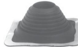
Suitable for extremely high and low temperature applications; service temperature range -100°F to 500°F. Works with any corrugated metal roof. Aluminum flanged base bends to fit irregularities. Forms watertight seal with proper sealant and standard fasteners. Includes clamp.
