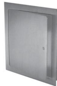
For installation in drywall, plaster, masonry or tile ceilings and walls. Features rounded safety corners, one-piece trim flange and continuous concealed hinge. 1-1/4" deep mounting frame with screwdriver-operated cam latch. Gray baked enamel finish.
