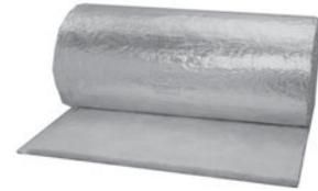
For use on ducts, pipes, return air duct pans, refrigeration equipment and crawlspaces, as acoustical insulation or water heater jacketing. Helps stop heat loss and provides barrier against radon and vapor. Lightweight. Resists mold and mildew. Environmentally safe; installation does not require respirator or protective clothing. Thermal rating of R-5.6 with spacer, R-4 without spacer. Meets federal and state building codes. ASTM certified.
