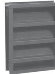
Features front flange; extruded aluminum 4" deep frame and non-adjustable 45° blades on 5" centers; 5/8" x .040" aluminum birdscreen on removable frame. Mill finish. Max. airflow 748 FPM; max. wind load 20 lbs./sq. ft.
