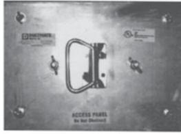
Sandwich design reduces installation time, eliminates need for welding and minimizes duct penetration. Grease-tight. Black iron construction. UL and CUL listed. Meets NFPA 96 standards.
