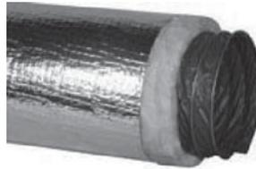
For low to medium pressure HVAC systems requiring mid-range sound levels. Manufactured to meet the highest quality standards in strength, permeability, and fire resistance. Fabricated with an acoustically transparent PE or CPE inner film which allows mid-range sound to penetrate the duct wall. Pressure rated to +10 and -5 w.g. (18" and 20" to -1 w.g.) Velocity rating 5500 FPM, Temperature range -20°F to 250°F, UL 181 Class 1.
