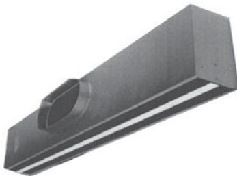
T-bar lay-in design for use in variable or constant-volume heating or cooling systems. 24-ga. steel construction with aluminum vane. Vane adjusts for left, right or vertical throw. 1-1/2" slot width. Black finish. **2-Slot.** Features black center tee.
