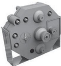
The CP101 pneumatic controller is the most versatile pneumatic controller available. This unique controller maintains the air flow dictated by the thermostat while compensating for changes in duct static pressure. The air flow control is pressure independent.
