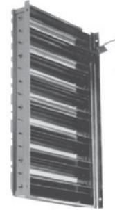
For use with square neck diffusers. Lever operated; blades regulate air-flow and ensure even air distribution. Steel construction with mill finish. Measures 2-3/8" D. Mounts directly to diffuser neck using sheet metal screws (not included).
