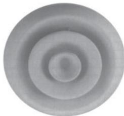
For heating and cooling applications. Three-cone design provides 360° horizontal discharge. Pattern can be altered by adjusting position of two inner cones; position 1 provides maximum capacity, while position 2 provides increased air induction. White.
