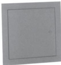
Provides service access to plumbing, heating, air conditioning and electrical systems. For use in masonry, tile or wood walls. Features 14-ga. steel door, 16-ga. steel frame with 1" flange, concealed hinges and screw-driver-operated cam locks.
