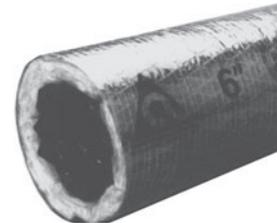
For use as supply or return duct in low to medium pressure systems, or as connection to mixing boxes, diffusers, room inlets or terminal devices. Features encapsulated steel wire helix core wrapped in fiberglass insulation blanket with puncture-resistant gray polyester jacket. 25-ft. length. Max. velocity 5000 FPM. R-value 4.2. UL 181 compliant.
