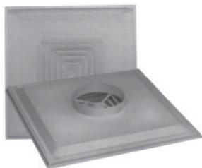
Generates high induction pattern for maximum throw at lower noise and pressure drop levels than curved-blade designs. Features heavy-gauge steel backpan with hinged perforated face (3/16" holes on 1/4" staggered centers). Airflow pattern can be adjusted for side or corner blow, horizontal or vertical. 24" x 24" flush face. White.
