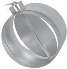
For use in low and medium velocity non-corrosive air systems. Features 20-ga. galvanized steel frame with pressed-in neoprene bearings; 20-ga. galvanized steel blade mounted to 3/8" square axle; quadrant locking handle on 2" standoff. Measures 9" L. Mill finish.
