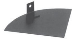
For closing off diffuser inlet quadrants to achieve specific air pattern. 90° angle; fits round neck diffusers. Steel construction with black finish. Installs inside diffuser neck using #8 sheet metal screw (not included).
