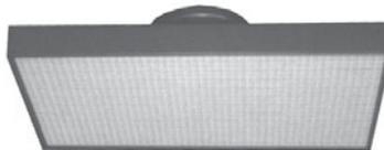
For lay-in installations. Features aluminum eggcrate grille (1/2" x 1/2" grid) with built-in 24-ga. steel plenum. 2-1/2" high beaded collar provides secure duct connection. White.
