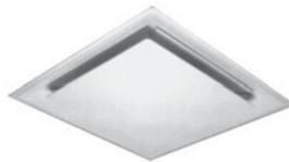
Features built-in heating and cooling thermostats, actuator and damper. Variable Air Volume design regulates discharge opening in relation to air volume, providing constant velocity, improved room air movement and uniform temperature distribution. Automatic changeover between heating and cooling modes. Temperature setpoint 70°F to 78°F; ±1.5°F accuracy. Diffuser measures 24" x 24".
