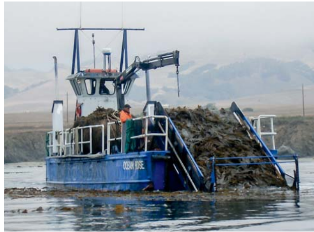
FIGURE 17.11 A kelp harvester designed with a mower on the bow of the vessel to remove the surface canopy of a giant kelp forest. Photo: Kendra Karr.
