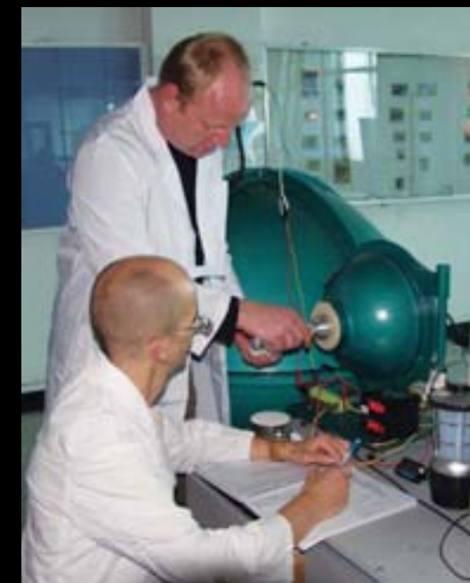
Lumens are measured in an integrating sphere, the most accurate device for measuring light output.
