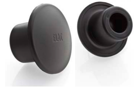
Bass control (BC) Polyethylene foam plug for bass reflex speakers with bass reflex tubes of 60 or 70 mm in diameter. The Bass Control plug closes the bassreflex vent and may compensate problematical acoustical circumstances, e.g. if the speakers have to be positioned close to the wall.
