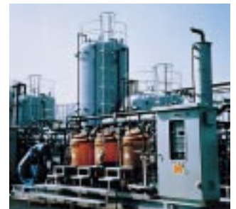
Model of Toray's new high-efficiency, two-step seawater desalination equipment at the Ehime plant
