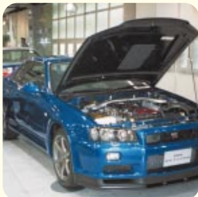
Torayca* is used for composite hood panels in the Nissan SKYLINE GT-R.†
