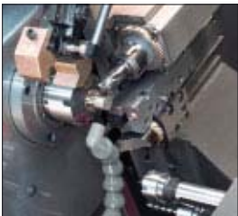
Back-operation machining Radial milling
