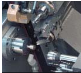
Turning using the HSK tool holder
