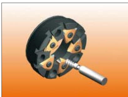
The defined thread length is reached. The Schwanog whirling spindle initially moves radially and then back axially. End of the whirling process.
