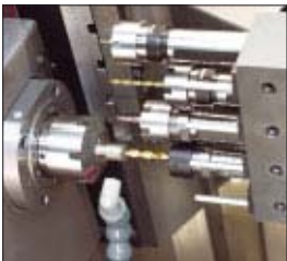
Back-operation machining End drilling
