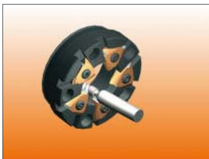
Thread whirling begins. The thread is manufactured by a rotating movement of the C-axis and a longitudinal movement of the Z-axis, and only one cutting edge of the whirling spindle is ever in use.
