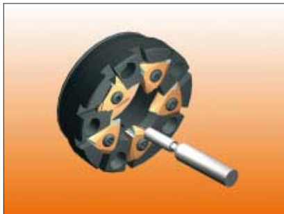
The Schwanog whirling tool is set-up in front of the workpiece and turns at high speed. The spindle and workpiece turn at lower speed in the same direction.
