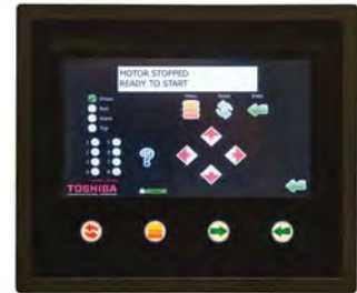
Touchscreen, showing previous keypad programming method/display.
