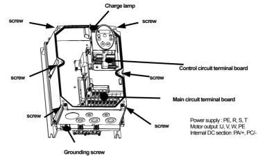
How to open the front and control circuit terminal (0.75kW – 7.5kW)
