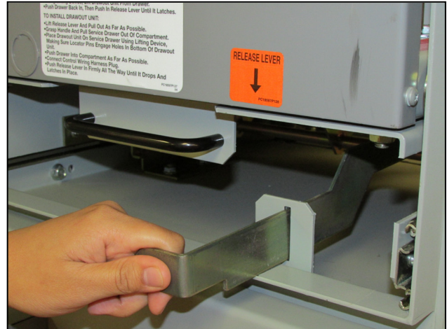
Fig. 21 Release Lever Pulled Out, Withdrawable Type Contactor
