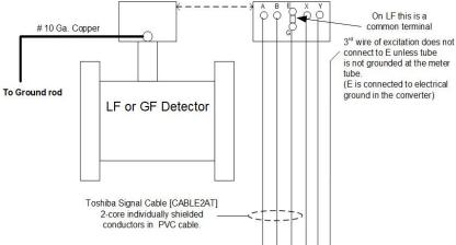
Magmeter connections for Remote Style Converters
