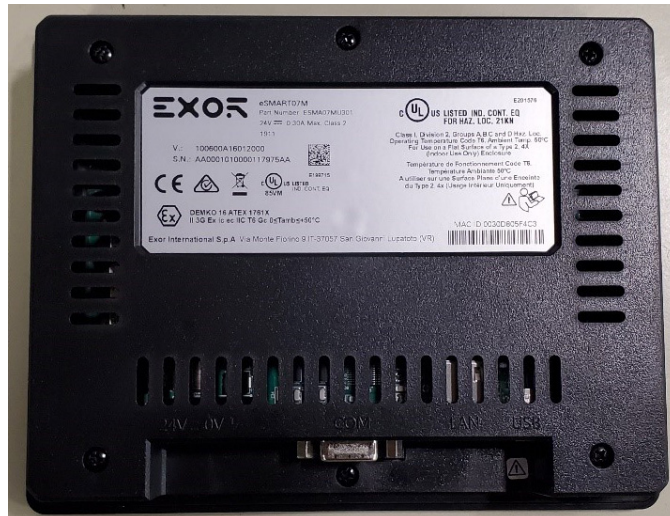
FIGURE 3.5: HMI SCREEN (200134), BACK VIEW
