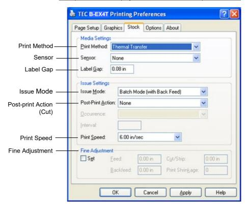
Print Method: Direct thermal or thermal transfer is selectable.
