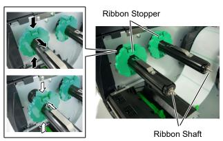
**2.** Leaving plenty of slack between the ribbon spools, place the ribbon onto the Ribbon Shafts as shown below.
