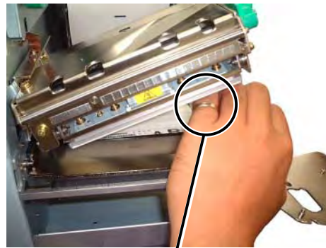
Care must be taken not to allow a metal object like a ring to touch the print head edge.
