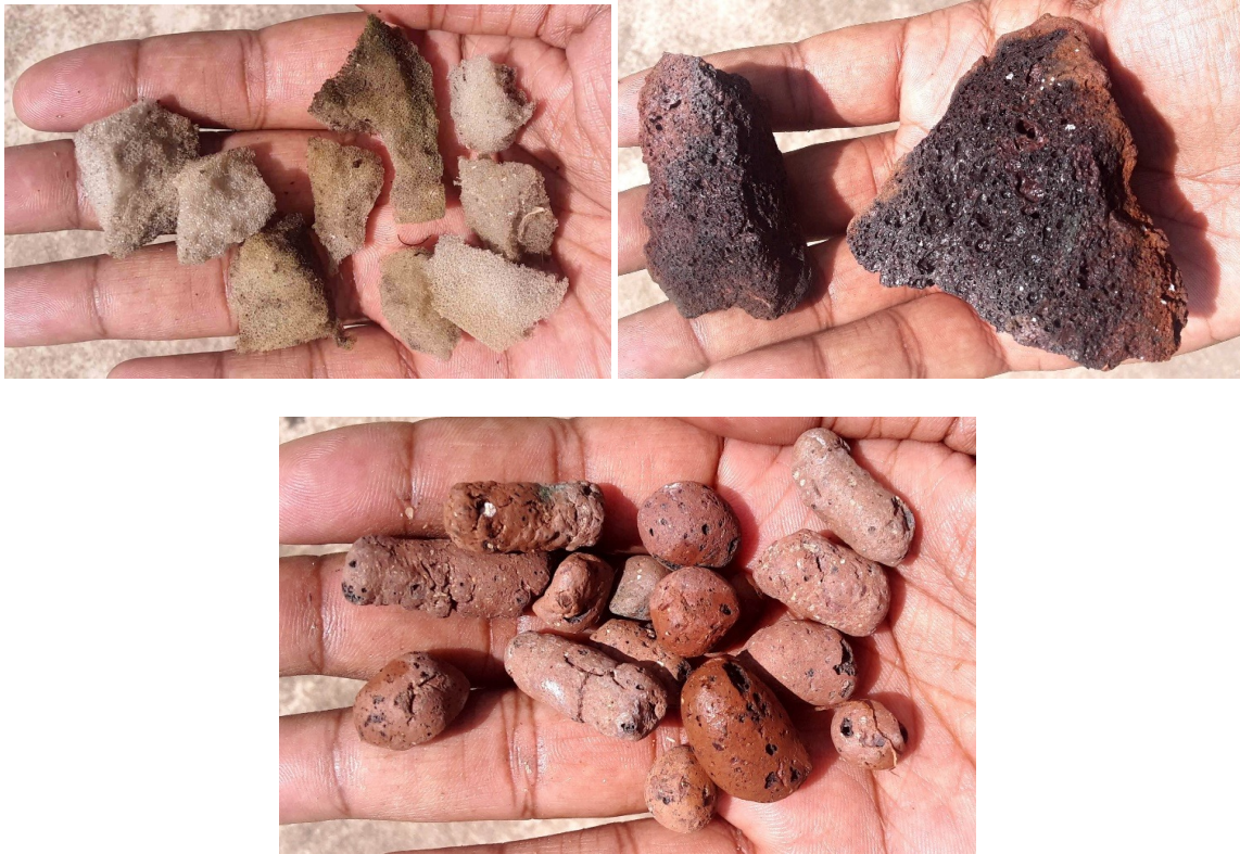
Fig 1, 2 & 3 showing Artificial Sponge pieces, Burnt Clay pieces and Hydroton Pellets
