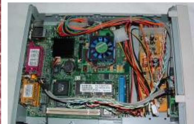
*The micro A1 installed in a Morex miniITX desktop case. The smaller board to the right is the power supply.*
