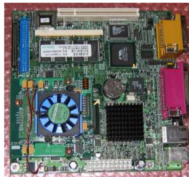
*The motherboard as it arrived. Notice the SODIMM memory module (with the white label) and the CPU module (with the fan).*
