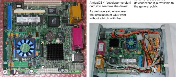
The motherboard as it arrived. Notice the SODIMM memory module (with the white label) and the CPU module (with the fan).
