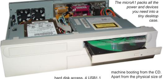
133MHZ, a Radeon 7000 graphics controller, a CMI8738 6 channel audio controller and a 10/100 3COM Ethernet
