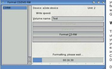
This new utility is used to prepare CDs and DVDs for on-the-fly reading and writing. Once a disc has been prepared it can be used just like a giant floppy!
