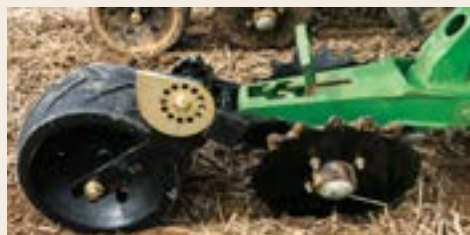
(Shown with (MRT800419) 6" rubber packing wheel and (MRT011344) dimple closing wheel set.)
