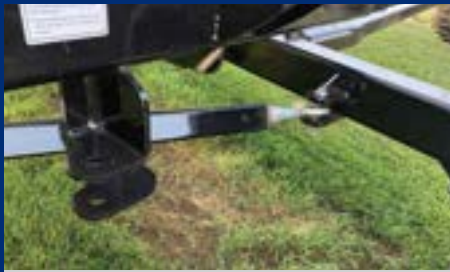
Crossover Tube Assembly Shown In Articulation Mode
