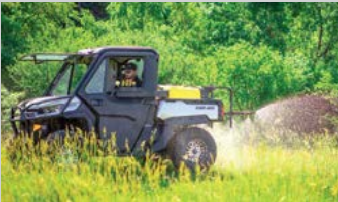
PROUTV65-12V-M with BXT3438 Boom. 65 Gallon with 12 Volt Pump, 3 Section Manual Control Arm with 25' Hose, Pro 22" Spraygun and BXT3438 Boom with 34' Coverage.
