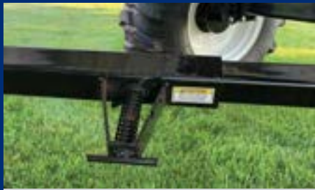
Snap Pin Used When Switching Between Transport & Articulation Mode
