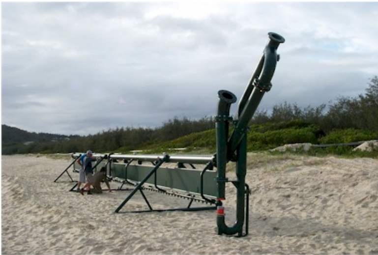
sand shifter unit: on the beach prior to deployment at the extraction site
