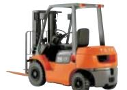
**7FGF/FDF25** Internal Combustion Counterbalanced Forklift Truck
