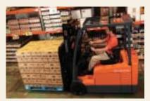
**7FBEU20** Three-Wheel Electric Counterbalanced Forklift Truck
