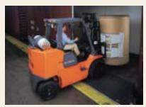
**7FGCU55-BCS**Internal Combustion Cushion Tire
