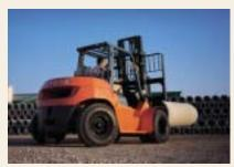
**7FGU70**Internal Combustion Counterbalanced Forklift Truck
