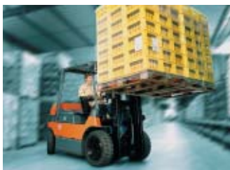
7FBMF45 Electric Counterbalanced Forklift Truck
