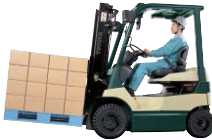
GENEO-B (7FB15) Electric Counterbalanced Forklift Truck
