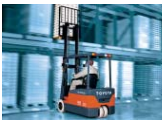
7FBF18 Three-Wheel Electric Counterbalanced Forklift Truck
