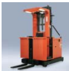
BT OPAL High-Level Order Picking Truck
