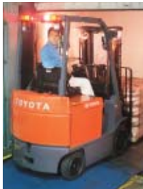
7FBCU25 Electric Cushion Tire Counterbalanced Forklift Truck
