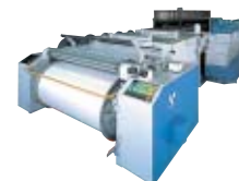
Filamaster Express 610 Sizing Machine for Filament Yarn
