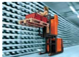
LOP10CF Low-Level Order Picker with Elevating Cabin
