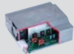
DC-AC inverter for the Tacoma (400W)
