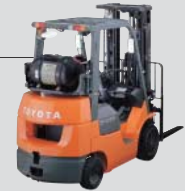
A compressed natural gas option is available for Toyota's 4,000-6,500 lb. internal combustion cushion and 3,000-6,500 lb. pneumatic lift truck models.
