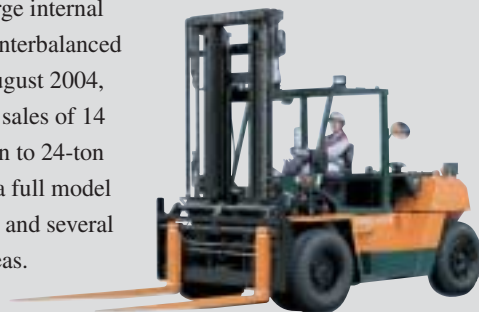
The series of 10- to 24-ton internal combustion counterbalanced lift trucks are the world's first models in their class to be fitted with a diesel turbo engine with a common rail direct injection system, achieving the highest level of power output, excellent fuel economy and clean exhaust emissions. They are also equipped with a highly durable 2-stator torque controller and efficient wet-type disk brake offering low maintenance and improved safety.
