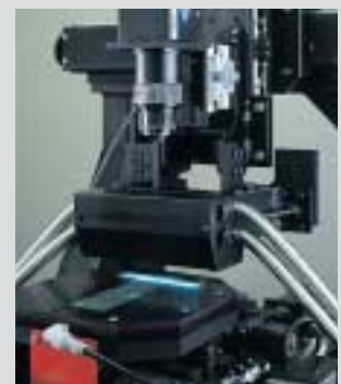
Circuit board inspection system with high-resolution line scan camera
