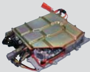
DC-DC converter for the PRIUS
