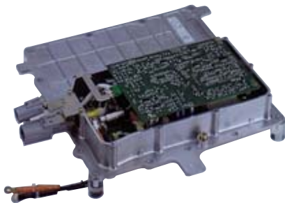
DC-DC Converter for the Prius
