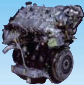
1CD Diesel Engine (Displacement: 2.0 Liters, Used in the Avensis and Corolla)
