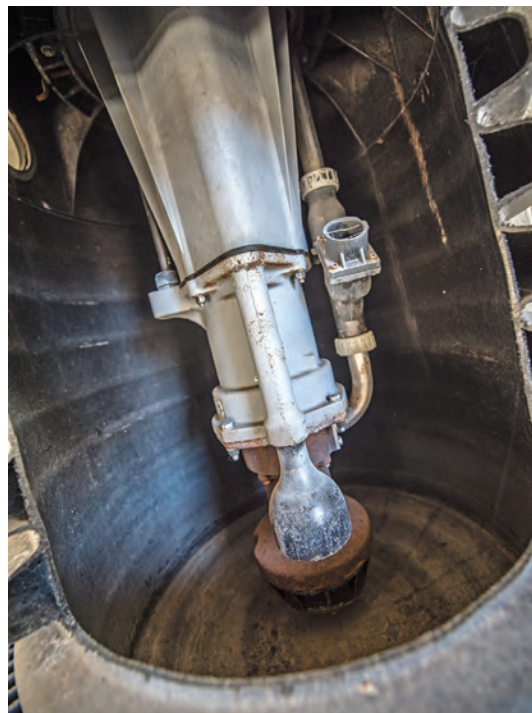
A cross-cut housing displays the workings of a grinder pump.
