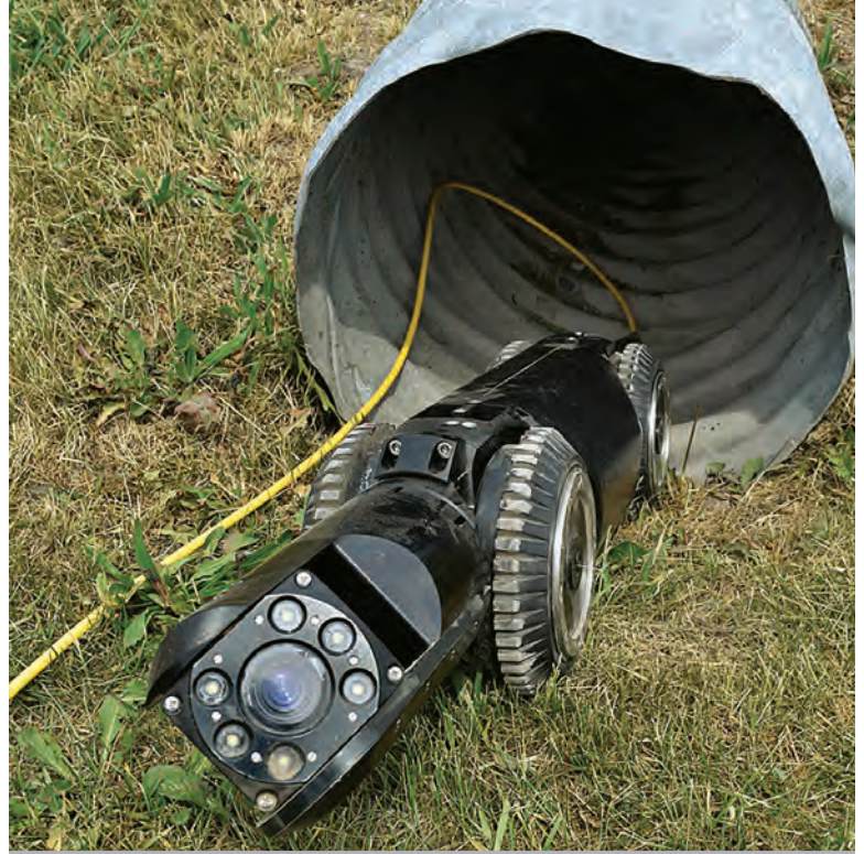
The crawler camera from Deep Trekker is operable by one technician and is fully submersible.
