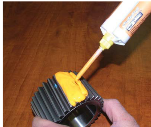
Shown Above: Quick Dispense internal casting (left) and external casting (right) using the new Flexbar Repru-Mix II Dispensing Gun System.
