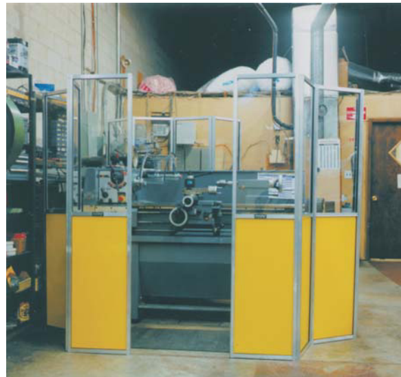
Shown above: Panelguards used to separate in-line machines. Protects operators from chips and noise from neighboring machines.
