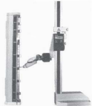
Calibration of Height Gauge using vertical position
