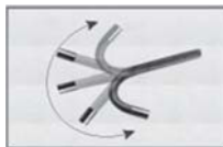
2 way articulation guides the viewer around corners and dark recesses.
