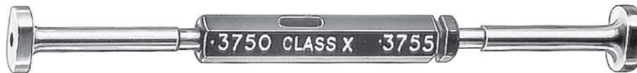
Gages up to 1/2" diameter are taper-lock type. Overall length of double ended gage is 3 1/2 inches.
