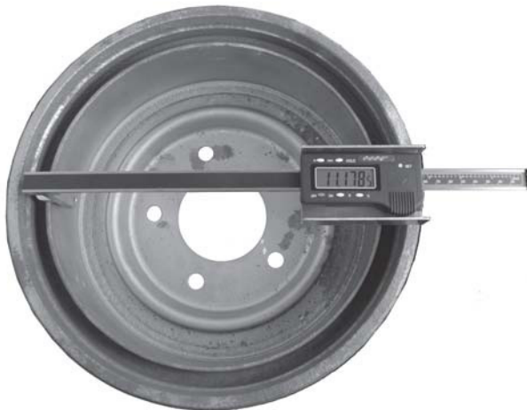
Shown Above: Internal Drum Diameter Measurement
