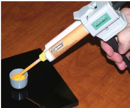
Shown Above: Quick Dispense internal casting (left) and external casting (right) using the new Flexbar Repru-Mix II Dispensing Gun System.
