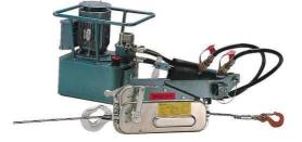
The TU-H Tirfor hoists are mechanically powered by a hydraulic cylinder using an electric or petrol powerpack. The TU-H adds flexibility to the operator particularly during extensive heavy-duty usage and movement of loads over long distances. Areas of application: maritime, building and industry, portable and flexible for use anywhere.
