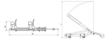
Fast and easy tensioning of wire ropes such as electric transport cables, telephone cables and fence assembly. Also suitable for pulling loads. Not suitable for lifting.
