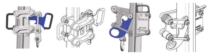
The Safety parking clamps (SPC) are dedicated to securing lifting platforms used in the elevator industry by attaching the platform to the guiding rail. They are used as a secondary safety device, a primary safety device is mandatory.
