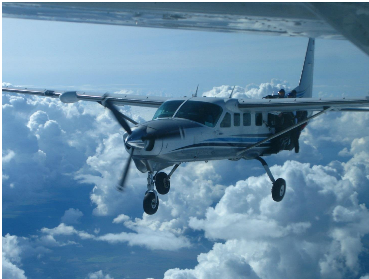
The centre of gravity shifts to the back. C-208 b D-FROB on the jump run. Pilot: Lasse Lintukangas. EENI 28 August 2010. Photograph by Antti Laukkanen.
