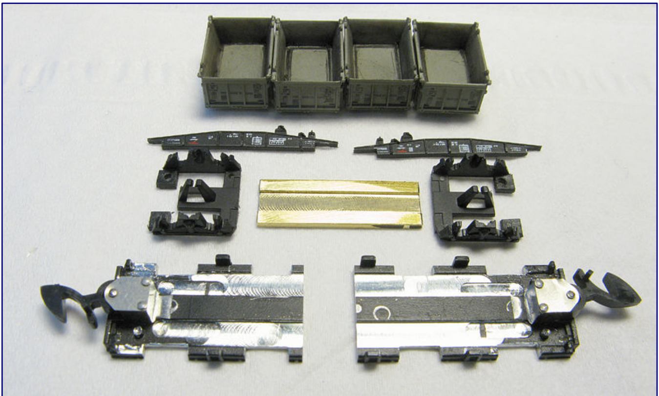
This photo of the dismantled trolley shows the cuts and milled parts required to modify the car into the missing desired model. A newly manufactured brass plate holds the chassis halves together in the future. Photo: Dirk Rohwerder
