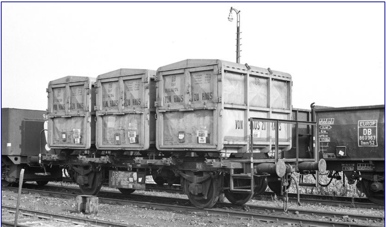
The container wagon BT 10 010 138 marks the new beginning and the expansion of door-to-door traffic driven by the German Federal Railway, based on the model from the Netherlands. The Ekrt containers loaded in August 1960 were built in this form in 1950 and belong to the original types of this system. When this photograph was taken in Braunschweig Rbf, the lashing of the Pa containers by eyelets on the wagon frame was no longer common practice. The advent of special containers meant that this form of transport securing was no longer possible. Photo: Reinhard Todt, Eisenbahnstiftung
