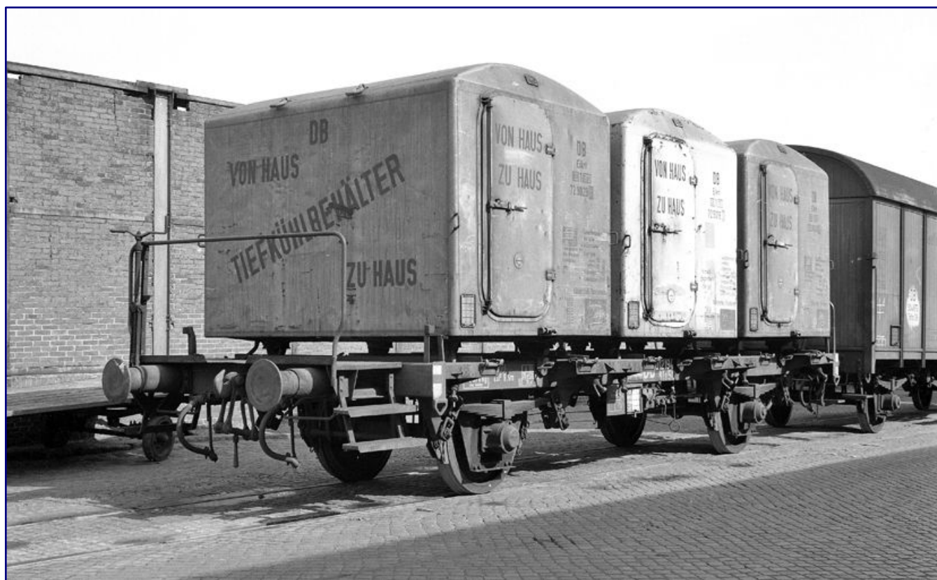
The comparison of the long side of this Pa container Eoskrt 021 with the Märklin model on page 6 reveals the differences in construction (top photo). The Eikrt freezer containers photographed in Braunschweig in September 1964 are among the first special types. Photos: Slg. Eisenbahnstiftung (top) / Reinhard Todt, Eisenbahnstiftung (bottom)
