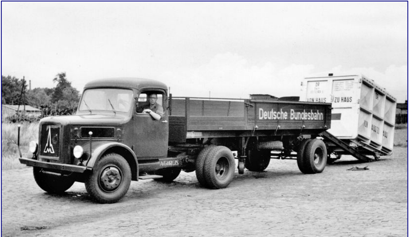
The simple semi-trailer shown here (German Federal Patent DE814275B), which accommodates a closed Ekrt container (built 1950) in 1951, was developed by the Bochum bus, bus trailer and vehicle manufacturer von Lienen and deviates considerably from the widespread Ackermann solution. Photo: Below, Eisenbahnstiftung
