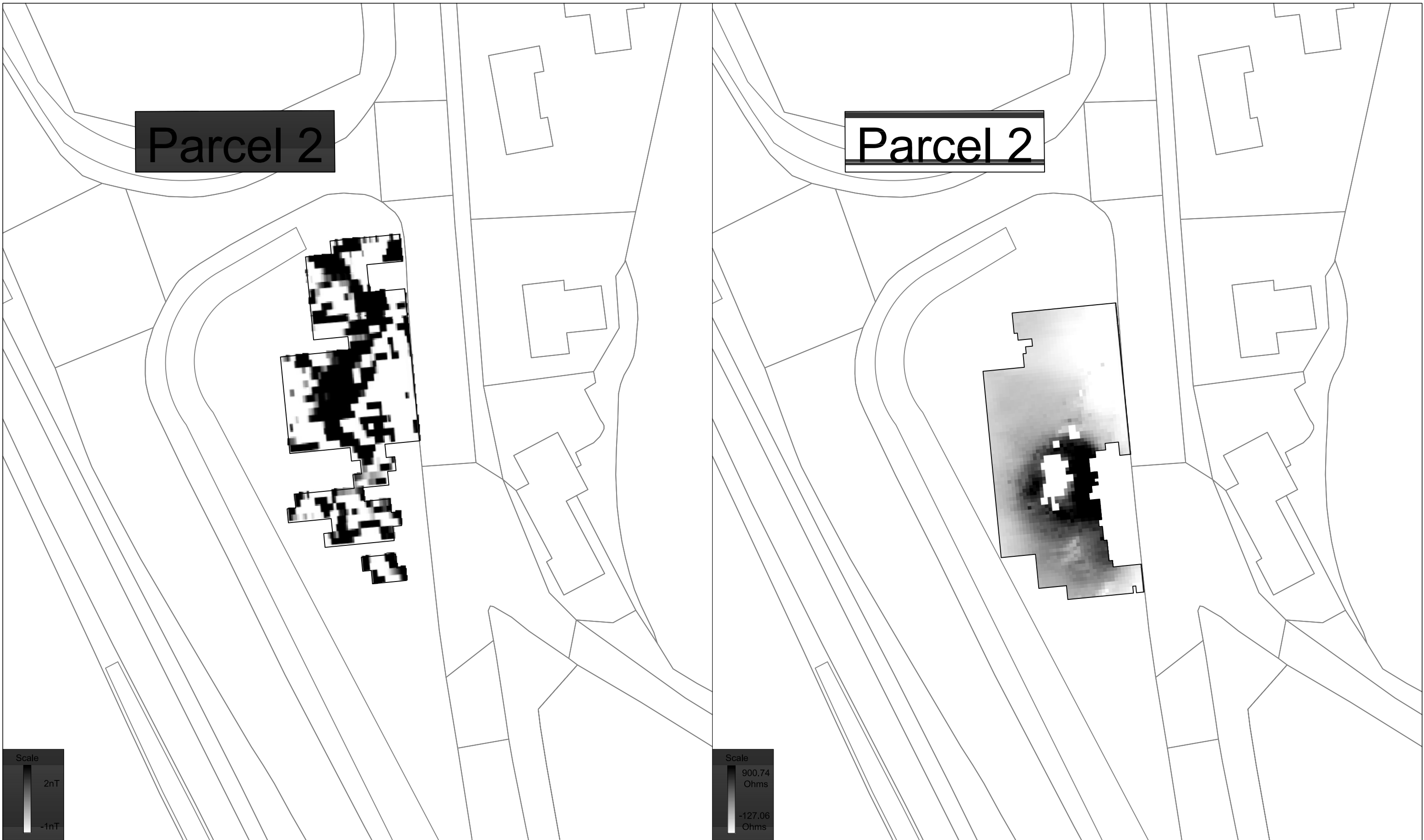
Minimally processed Gradiometer survey results - Greyscale plot - Parcel 2
