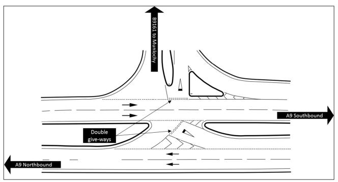
Figure 7-1: Existing layout of the A9/B9161 junction (Munlochy Junction)
