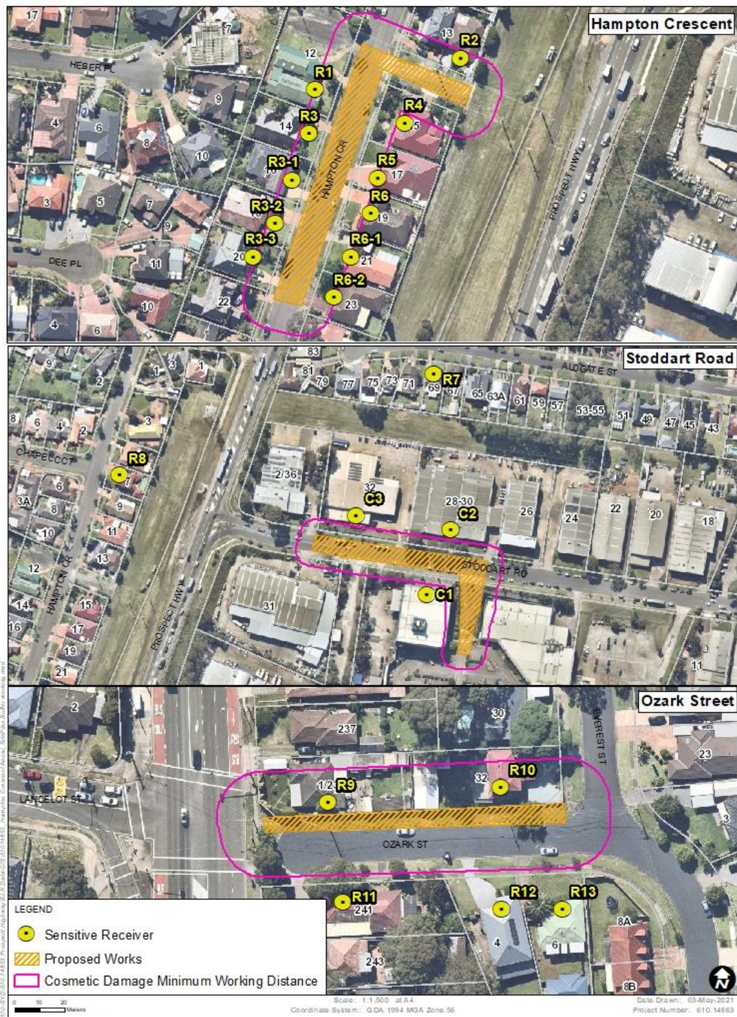
Figure 5 Vibration Assessment – Minimum Working Distances (Vibratory Roller)
