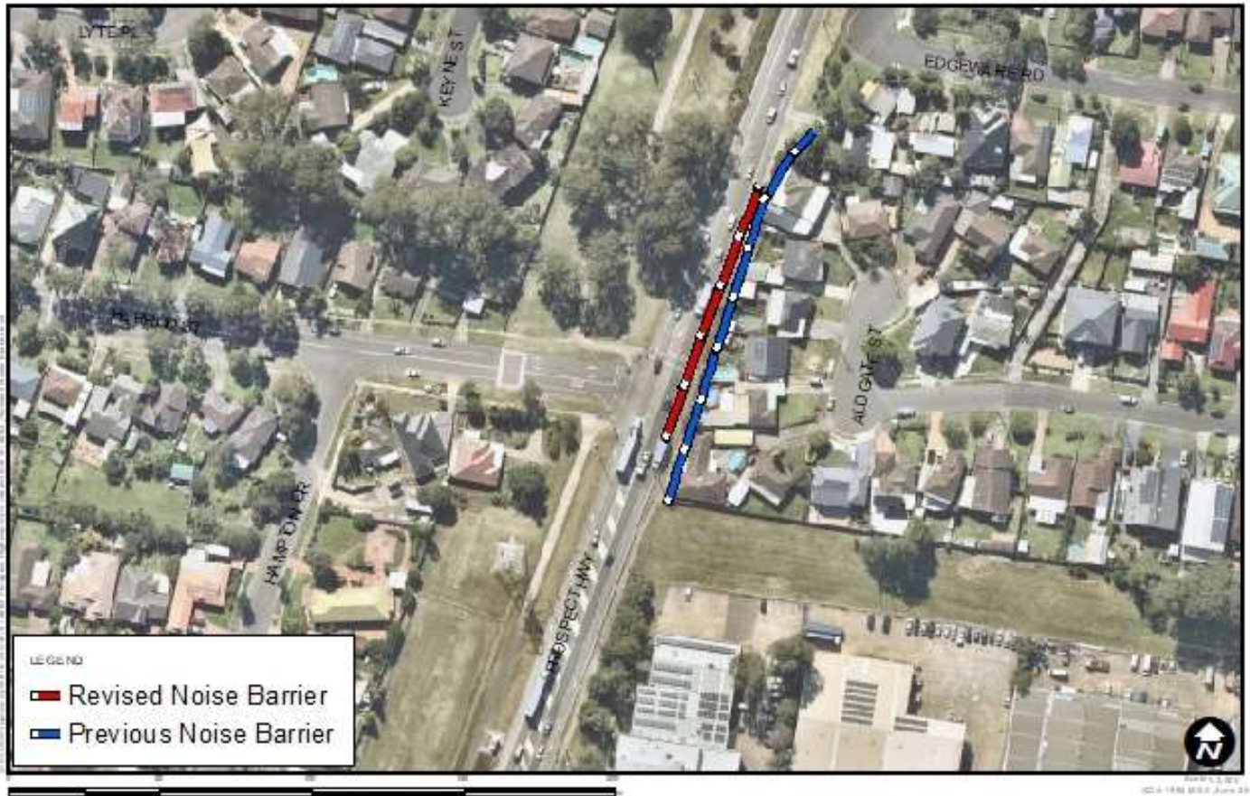
Figure 6-1 Revised noise barrier SB01
