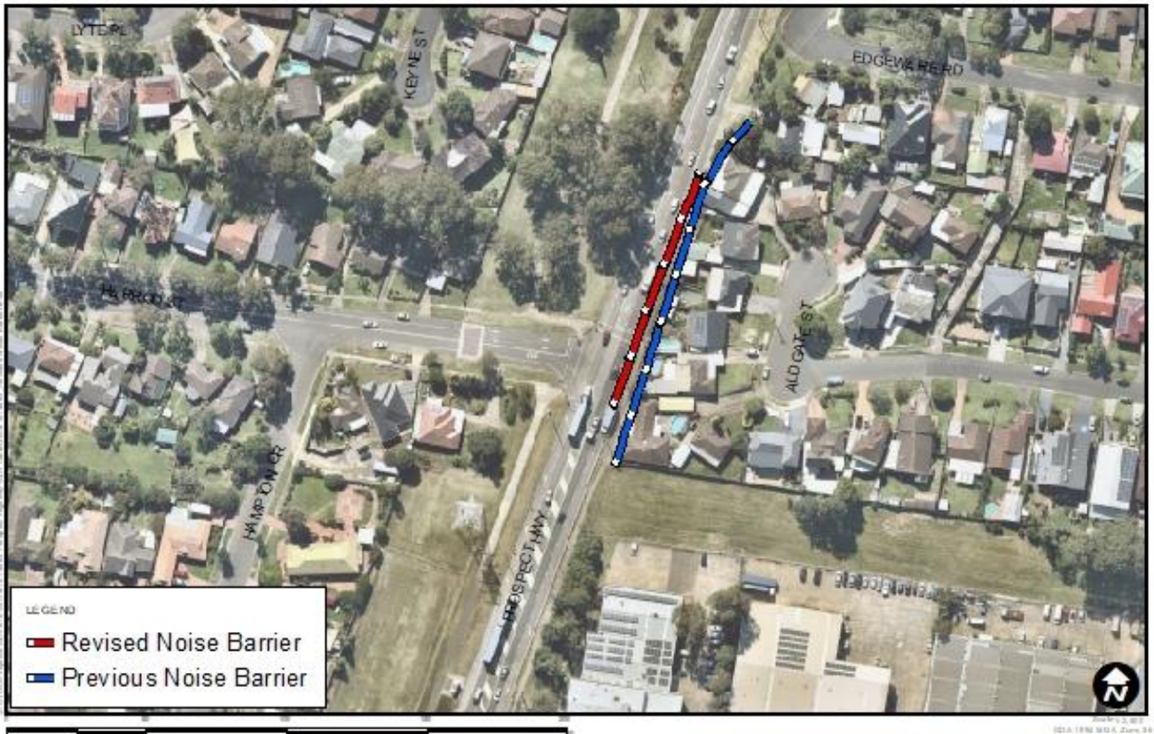
Figure 1 Alignment of New SB01 Barrier
