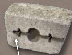
Closed end of receiving channel
